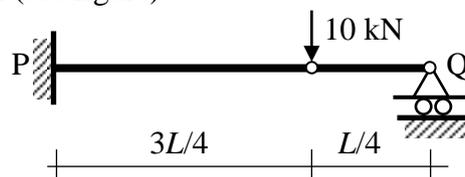
The vertical reaction at support Q is
