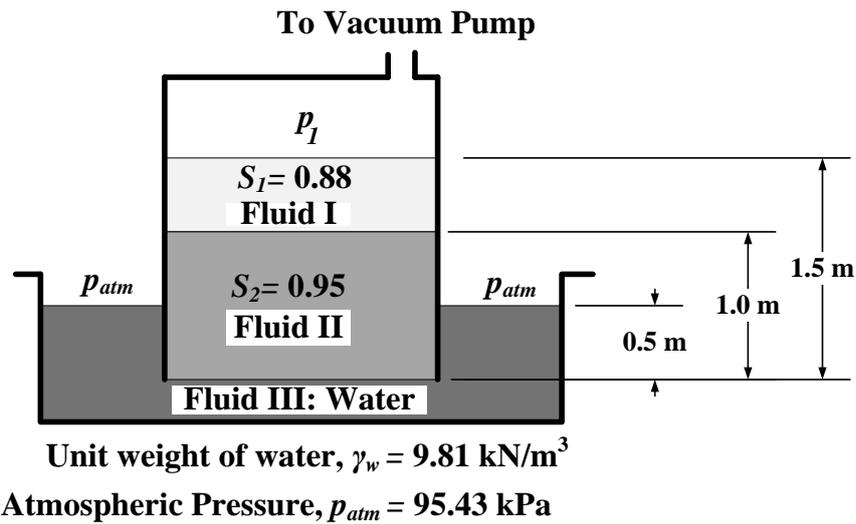
The gauge pressure value (in  $\text{kN/m}^2$ , up to two decimal places) of  $p_1$  is \_\_\_\_\_
