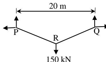
Neglecting the self-weight of the cable, the tension (in kN, in integer value) in the cable due to the applied load will be \_\_\_\_\_
